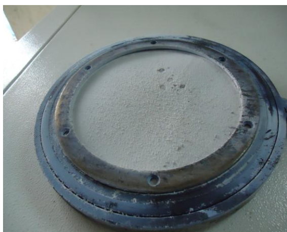
Figure 3 –Sample collector with glass fiber filter paper holder.
